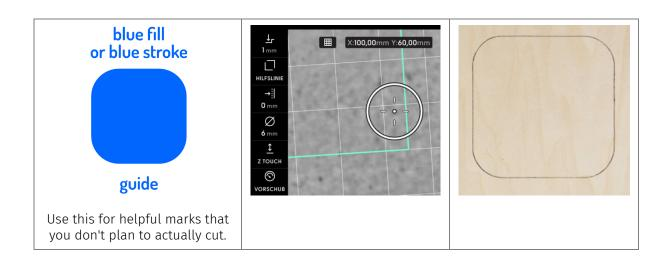
**Open shapes** (eg: a single, open-ended line) can be coded as a guide or online cuts. When cutting, Origin will center the cutter on the path.
