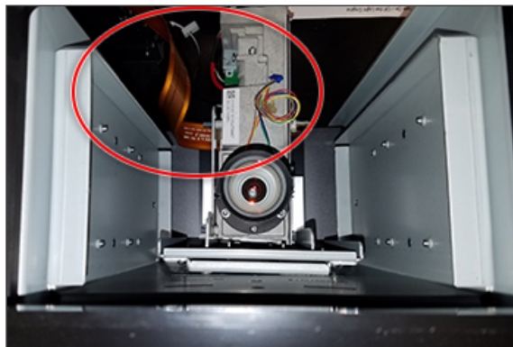
Visible wiring in bottom of build chamber, taken through view box.
